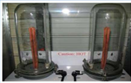
New heating elements in stand before test
